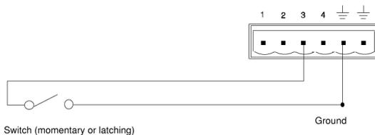
Figure 15: MUTE CONTROL PIN CONNECTIONS
