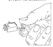
Grasp molded housing of stylus and gently pull forward out of cartridge. Insert replacement stylus into socket and press until housing mates with cartridge case.
