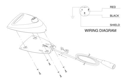
FIGURE 3: REMOVING THE BACKPLATE
