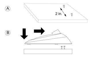
FIGURE 1: SECURING THE A412B TO A MOUNTING SURFACE
