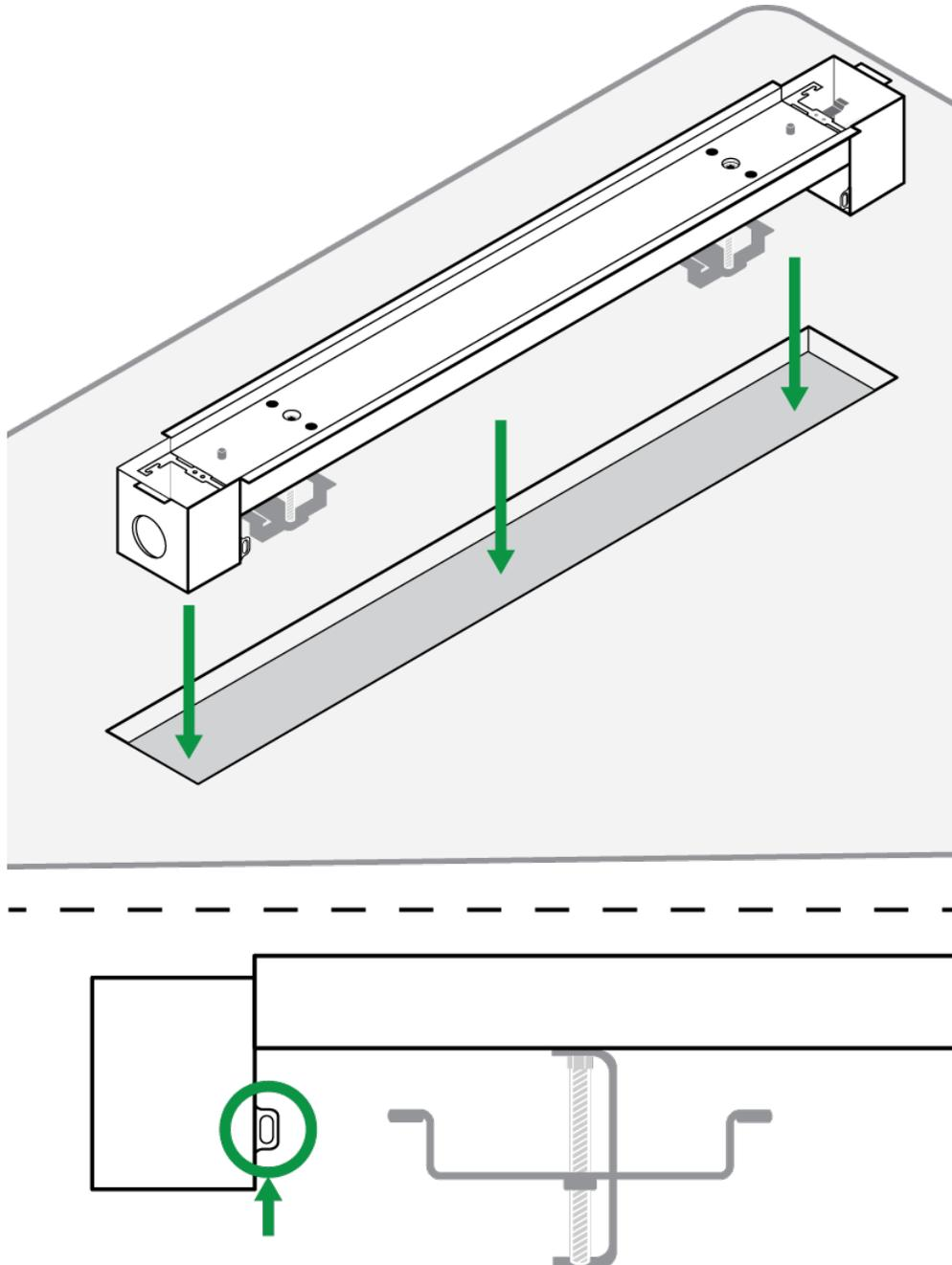
3. Tighten the 2 screws until the flush mount is securely attached. As you tighten the screws, the clamping brackets rotate to hold the flush mount in place.
