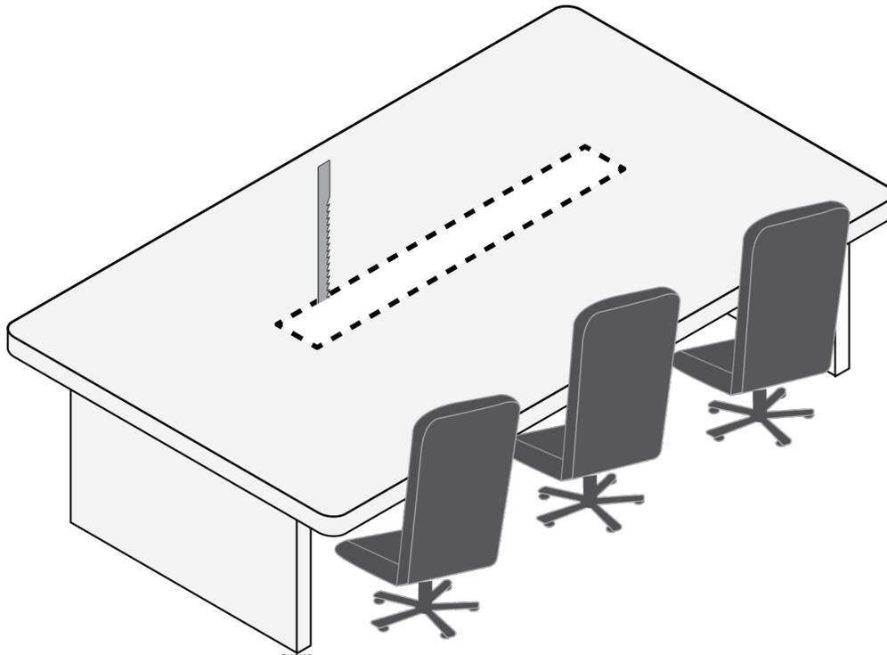
2. Place the flush mount in the opening. The clamping brackets should be parallel to the flush mount.
