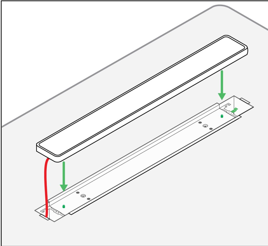
6. The flush mount frame has 4 clips that fit into slots at the corners of the flush mount. Squeeze each clip to fit it into the slot. It's easiest to hook one side of the clip into the slot at a time.
