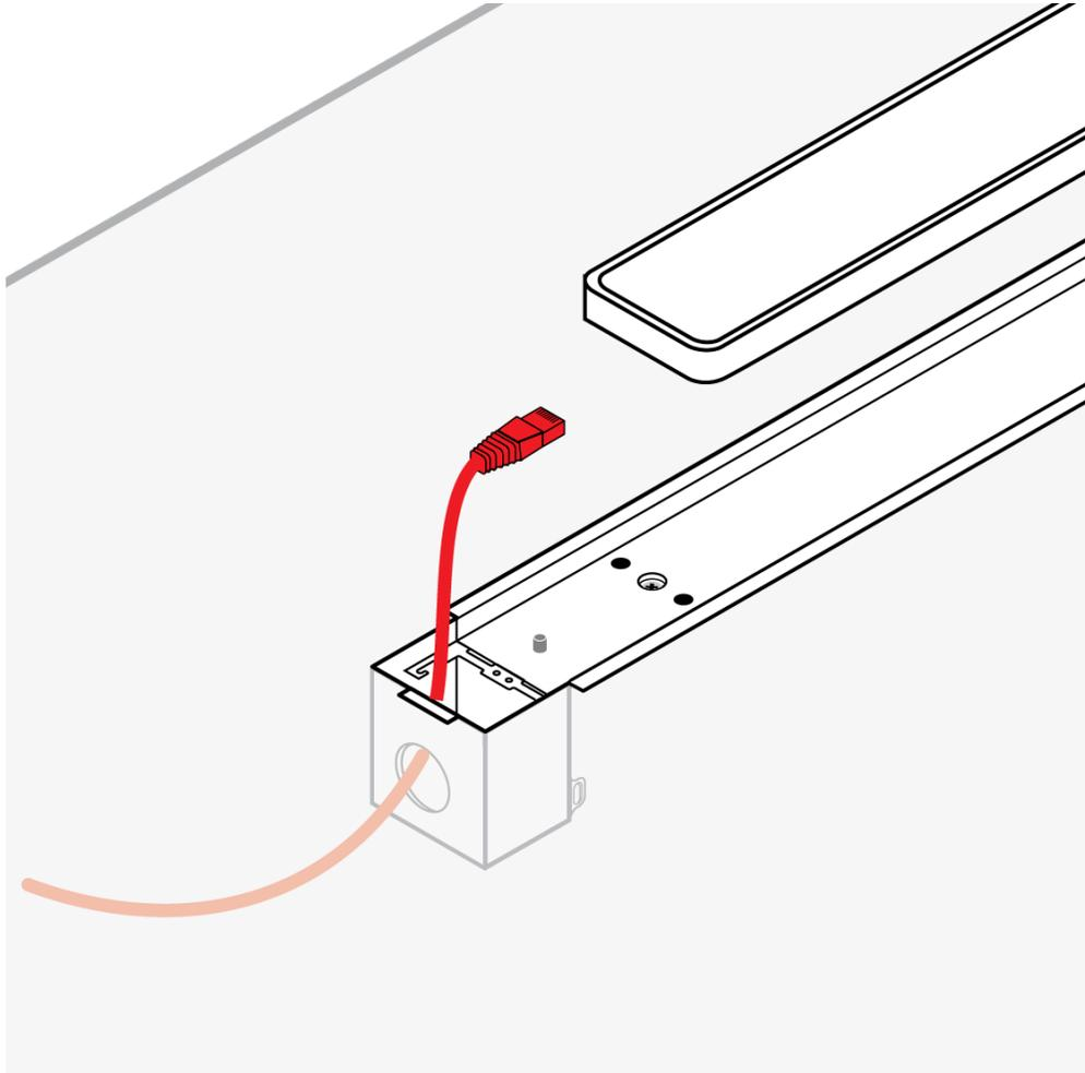
5. Align the holes on the bottom of the microphone with the raised posts on the flush mount. The metal tab on the flush mount also aligns with a square cutout on the bottom of the microphone. Place the microphone in the flush mount and slide it into place.
