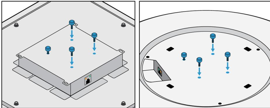
5. Lift the microphone and align the thumb screws with the holes in the VESA bracket. Tighten the thumb screws to secure the microphone to the VESA bracket.
