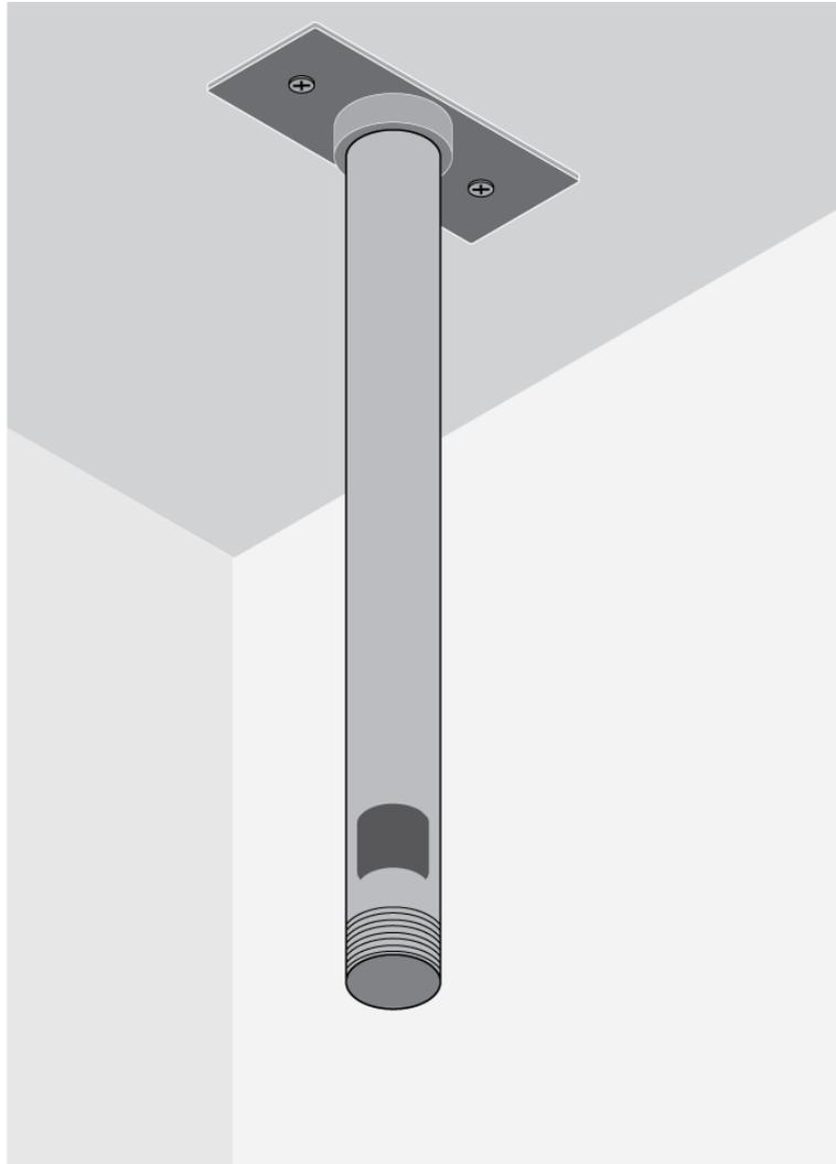
3. Thread the VESA bracket onto the pole.
