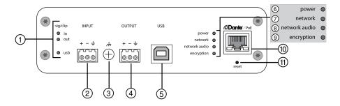
The LEDs on the front of the ANIUSB-MATRIX behave the same as the ones on the back of the device.
