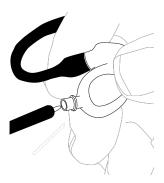
Caution: When cleaning, do not force any object through the earphone nozzle! This will damage the earphone sound filter.
