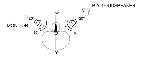
**Recommended Loudspeaker Locations for Supercardioid Microphones**
