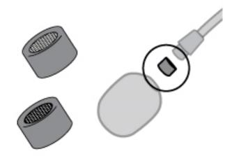
Always use the BETA54 with the standard protective cap only. Using the microphone with no cap, or with the filtered cap, will degrade sound quality and alter the microphone's polar pattern.
