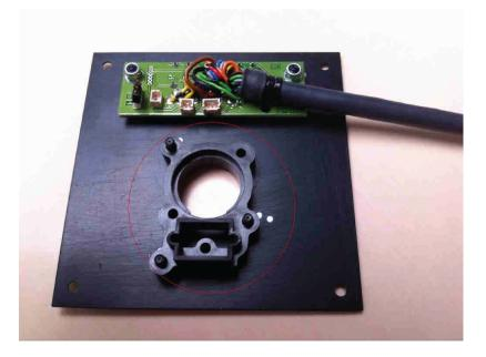
Step 8: Now insert the boundary mic into the sleeve of the XLR chassis and then tighten the 3 Allen screws on the bottom of the mic; this will cause the mic's rubber sleeve to expand into the XLR chassis and hold it in place. Connect the boundary mic to the PCB.
