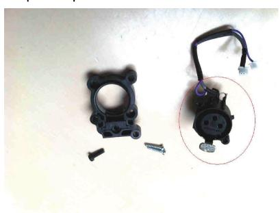
Step 5: Remove the plastic "lock" insert.
