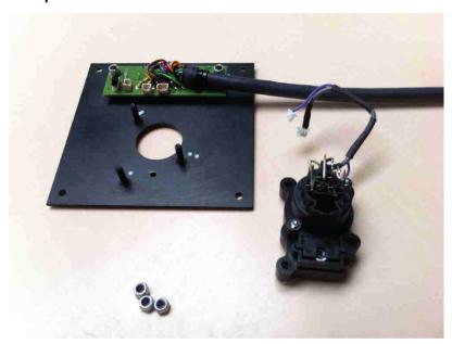
Step 3: Turn over the XLR. Undo and remove the two T8 torx screws and the 3mm Allen bolt.
