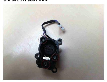
Step 4: Separate the connector section from the XLR chassis.
