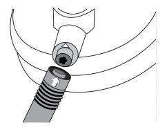
Attach the cable by aligning the arrows and pressing firmly into place until locked.
