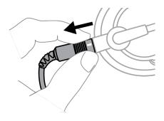
Pull on the knurled collar to disengage lock and remove cable.
