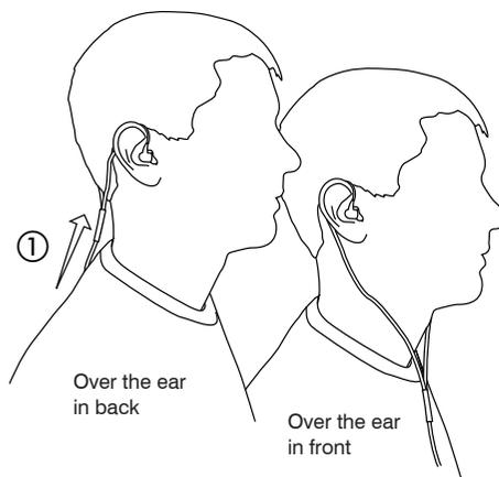
Tighten the cable and take up slack by raising the cable sleeve ①.
