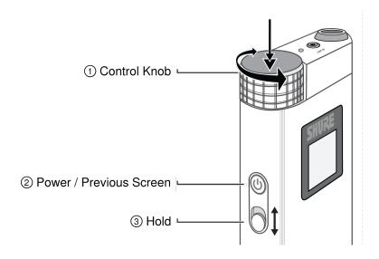
Powering on / off: Long press the power button ②
