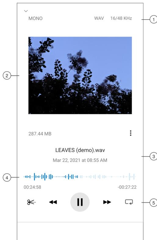
① **Track Information** Displays the name of the currently playing track, including file format, bit depth, sample rate, and stereo or mono.
