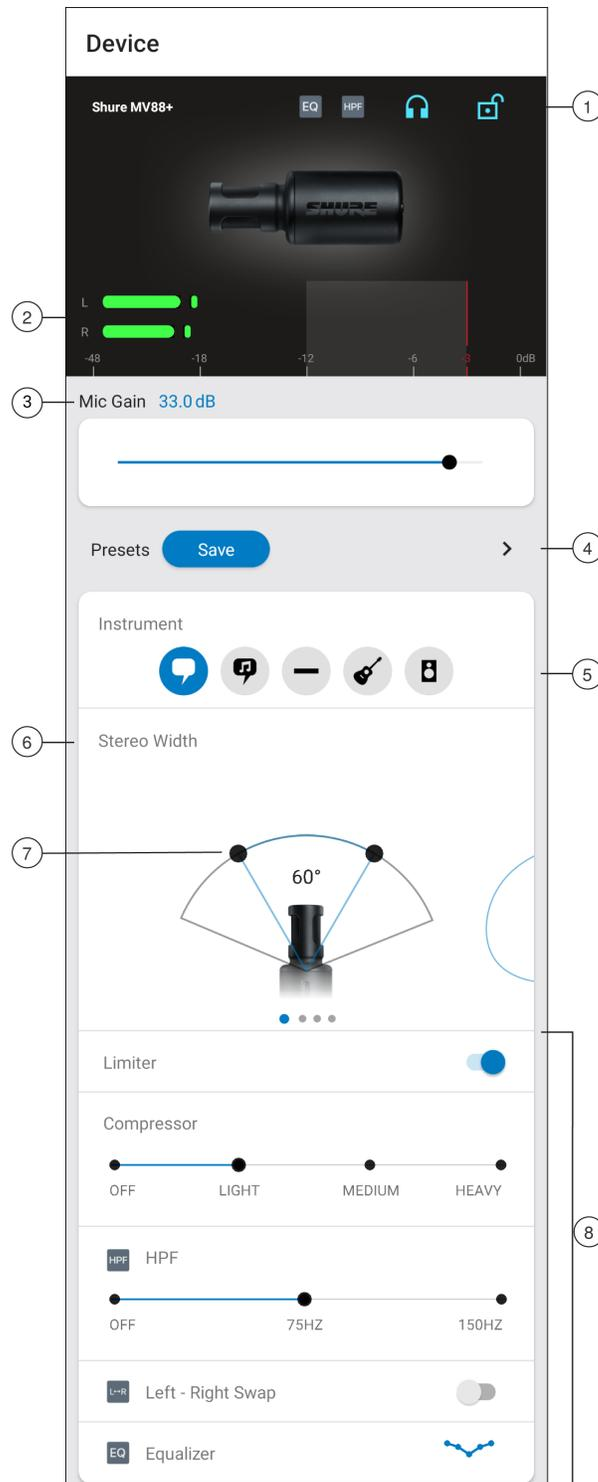
① **Notifications** The top row displays which device is connected. A red flashing dot next to the name let you know whether recording is active. The charms show which advanced features are on. Tap the headphone icon to access direct monitoring control. Tap the lock to lock or unlock the settings.
