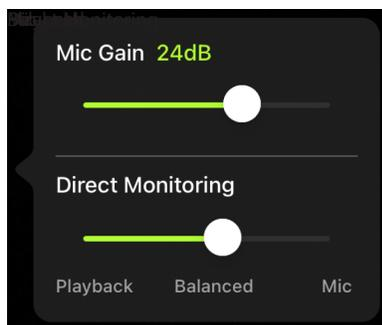
Use the direct monitoring slider to determine how much of each input you hear. For best results, start monitoring at the mid-point and adjust.
