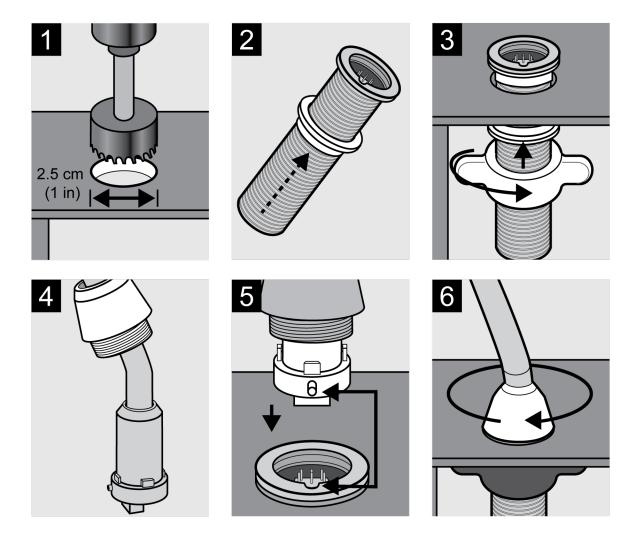
**Note:** Over tightening the wing nut reduces shock isolation.
