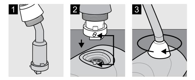
Caution: To prevent bending pins, line up key with notch and seat connector fully before twisting to lock.
