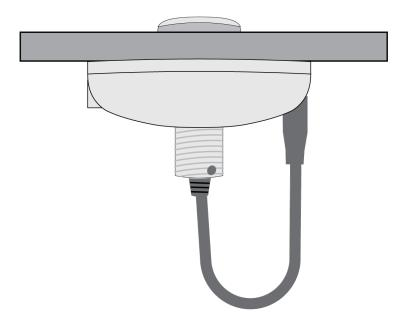
6. Connect a Cat5e (or better) Ethernet cable to the network port. Make sure the cable supplies Power over Ethernet from a network switch or PoE injector.
