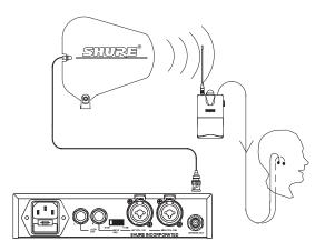
**Note:** Using too many transmission antennas in one installation can reduce performance. To combine PSM antennas, use a PA821 Antenna Combiner.
