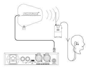
1. Determine the length of cable required to connect the PA805 Antenna to the Wireless Transmitter or Antenna Combiner. Use only as long a cable as necessary, because there is more power loss with longer cables.
