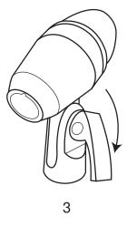
**Note:** To adjust the tension on the lever, pull it open and use a flat head screwdriver to tighten or loosen the bolt on the opposite side.
