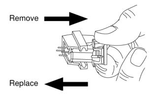
Remove and replace the stylus as shown above. Always hold the stylus by the plastic grip. Do not touch or damage the diamond tip or cantilever. Do not force.
