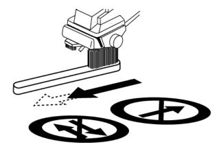
Use a soft brush with alcohol or an alcohol-distilled water solution. Commercial cleaning solutions may cause stylus damage. Brush only from back to front as shown here, never front to back or side to side.
