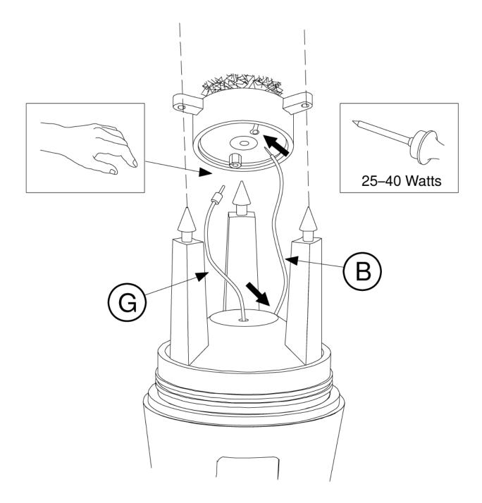
**IMPORTANT:** Once you have installed the cartridge, take care to position the blue and green lead wires so they do not touch each other, the cartridge or any other part of the microphone. Otherwise, noise problems may occur.
