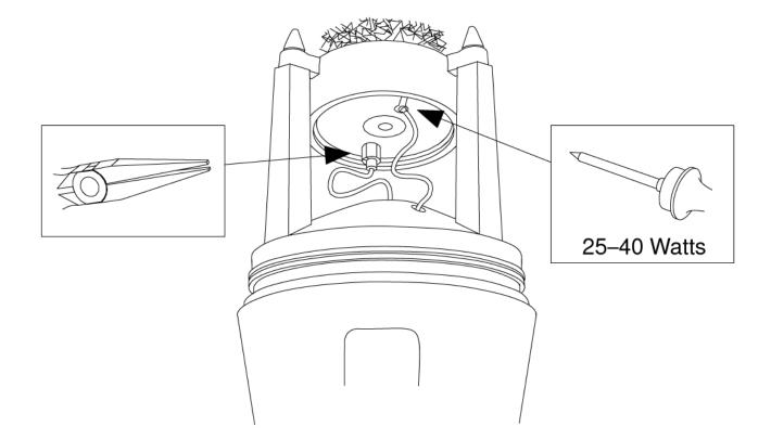
3. Remove the old cartridge by pulling off the rubber loops from the three shock-mount posts.
