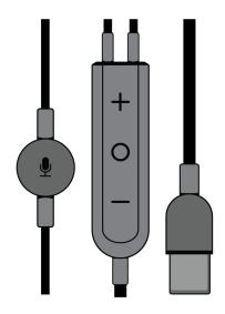
Shure USB-C cables are designed for continued functionality between mobile devices and your Shure earphones and headphones. They feature a USB-C connector and three button controls with in-line microphone for phone calls and voice applications.
