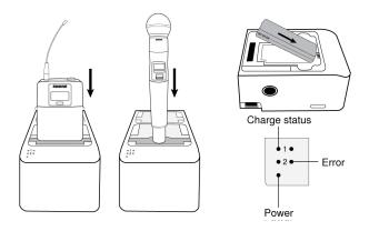
Warning: Do not insert transmitters using AA batteries.
