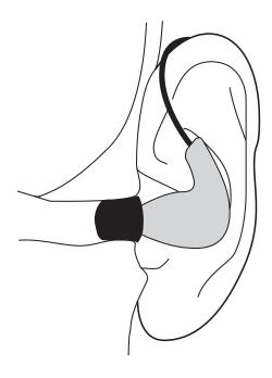
**Important:** If there seems to be a lack of low frequency response (bass), this means that the earphone sleeve is not forming a tight seal. Gently push the earphone deeper into the ear canal or try a different sleeve.
