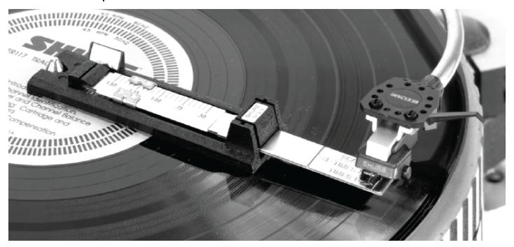
The Shure Model SFG-2 Stylus Tracking Force Gauge is a highly accurate beam balance that is designed for measuring stylus tracking forces from 0.5 to 3.0 grams in .05 gram increments. Its rolling bearing pin pivots are engineered for minimal friction. Each SFG-2 Tracking Force Gauge is factory calibrated.
