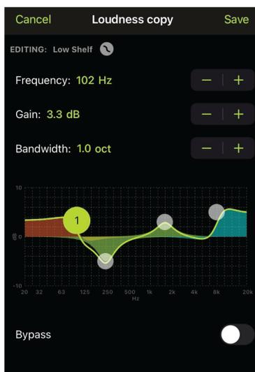
Select and adjust frequency, gain, and bandwidth in the equalizer.
