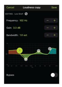
Select and adjust frequency, gain, and bandwidth in the equalizer.
