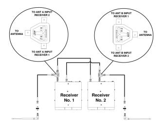
In this configuration, use UA221 or UA221Z, or ensure the receiver's DC bias is disabled.
