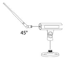
2. Use low-loss coaxial cable (sold separately) to connect to the receiver (or antenna distribution system), as shown.
