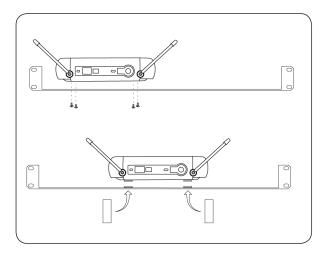
Use screws for installation if unit will remain mounted.
