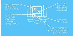
3-Lead Stereo Connection: When a 3-lead stereo input system is used, the common lead should be connected to both of the ground terminals at the cartridge. This connection should be made before connecting the regular terminal jacks to the cartridge. No other common ground connection should exist.
