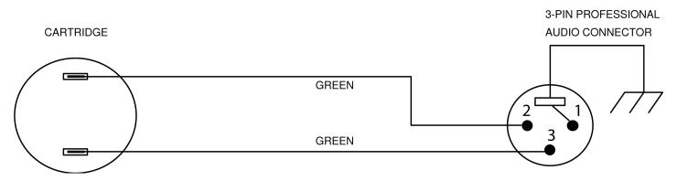
Figure 2: Internal Connections
