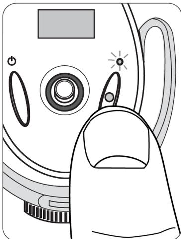
**Record:** Press the record button to begin recording. The LED indicator illuminates while recording. Pressing record always creates a new track, unless resuming a paused recording.
