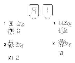
If setting up additional systems, leave the first transmitter and receiver on. For each additional receiver, manually set the group to match the first receiver. Note: The receiver will automatically perform a channel scan to find an available frequency after the group has been selected. Set the transmitter frequency to match the receiver.
