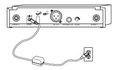
b. Connect receiver to mixer or amplifier. Press the power button to turn on the receiver.
